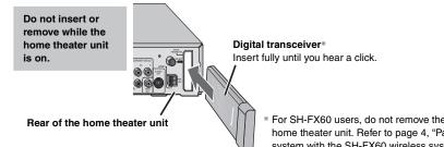
For SH-FX60 users, do not remove the SH-FX60T transceiver card from the home theater unit. Refer to page 4, "Pairing your SB-FX80 wireless sound system with the SH-FX60 wireless system (not included)".
