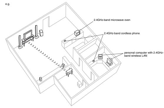
The wireless sound system will automatically seek a clear channel if any of these other devices interfere with its communication. When this happens, the wireless link indicator (e.g. " $\overline{W}$ " or LED) flashes on your home theater unit, and there is a brief interruption in audio coming from the wireless sound system.
